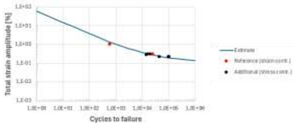
Figure 1: Material strain-life curve for C45E estimated with STEP
