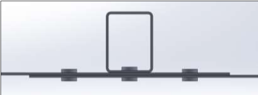
Figure 2 - Lap splice joint with tube section stringer
